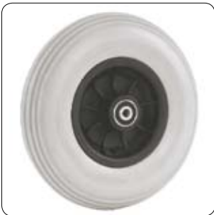
8" (200 x 50 mm) wheel with closed rim and ribbed polyurethane tyre
