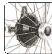
Hub with brake plate, QR axle and brake lever
